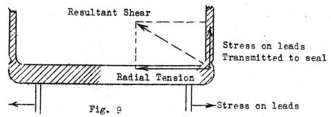
It is obvious that both seal and button strains act together to produce failures. The actual failure may occur in either member, depending on the location of the largest strain and on mechanical weaknesses.
