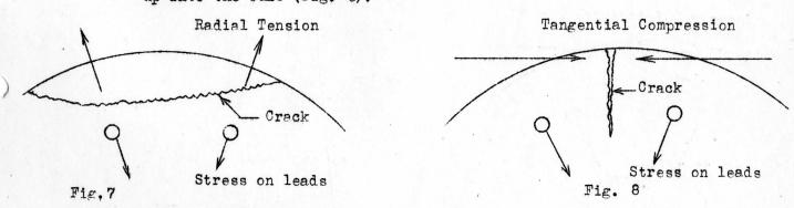
Most of the failures encountered belong to one of these (3) types. Cracked tubes returned from the field still have their leads bend outward, or in some cases, inward. This indicates that the sockets in use bend the leads, causing a stress on the glass.
