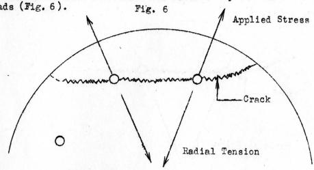
There will be an equal but opposite stress at right angles to the radial tension. This tangential compression will be decreased by an outward force on the leads.
