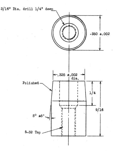
Model No. 786-J Part No. A-92 Made of stainless steel 3/8" diam. 5/8" lgth. 9805-R1
